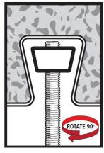
Rotate the rod assembled with the Wedge Nut at 90° making sure the tapered faces of the Wedge Nut are now facing the rib profile
