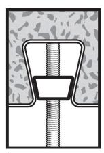
Rotate the threaded rod in to the Wedge Nut so that the rod touches the top of the rib (Finger tight). Check the tapered faces of the Wedge Nut touch the faces of the rib profile
