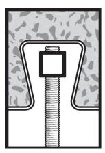
Attach threaded rod to Wedge Nut. Align parallel faces of the Wedge Nut along the length of the rib opening and insert all the way into the wider section of the opening
