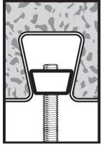
Pull down on the threaded rod so that the Wedge Nut tightly fits / seats in the rib opening of the BONDEK® profile.
